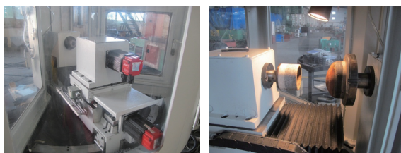
图8 离线气囊修整装置 Fig.8 Off-line dressing equipment of bonnet polishing head
